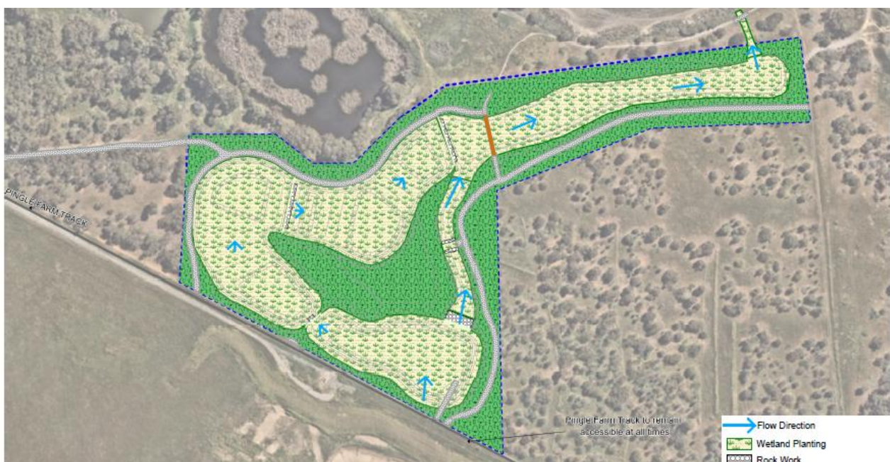
Figure 13 – Stage 4 – Minor earthworks – The Application Area will be prepared for plantings for water loving plants (yellow and green) and the surrounding terrestrial plantings (darker green). The brown line indicates the footbridge and grey the walking trails. The blue arrows show the direction of the water flow from the housing development Sunset, Port Noarlunga South through the wetland toward Ngangkiparri. Image: Hickinbotham Developments.
