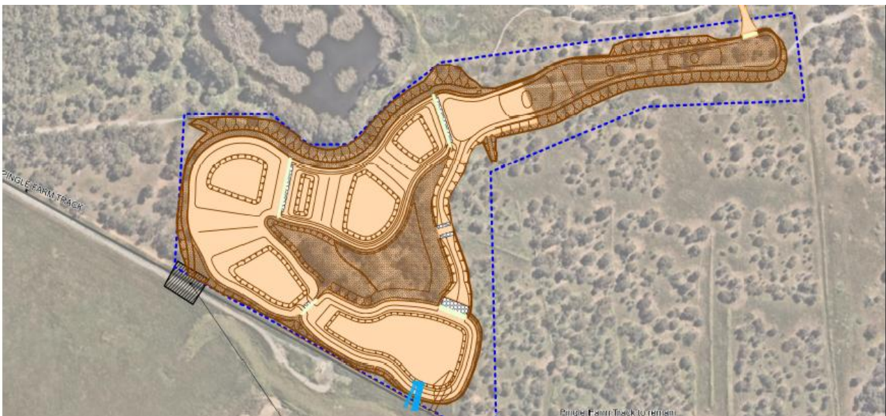
Figure 12 – Stage 3 – Infrastructure installation – A concrete channel (culvert and headwall in blue) will be built to funnel water underneath the road to the wetlands. Additional rock work (mottles) will be installed to prevent erosion of the water basin walls, weirs - concrete or rock barriers (pale green) - will be installed to manage water flow and factory-made liners (pale brown) will keep moisture in the basins to support plant growth. Image: Hickinbotham Developments.
