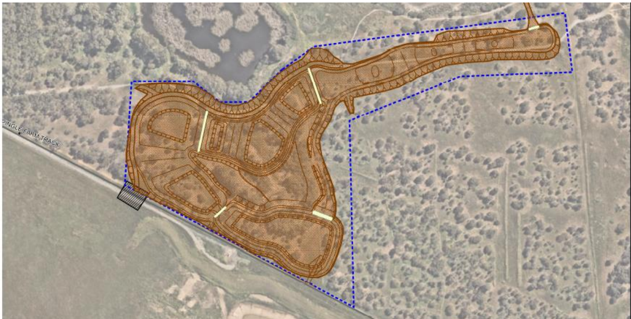
Figure 11 – Stage 2 – Earthworks and Excavation - The ground disturbing works are shown in brown with dark brown mottles indicating the location of rock walls to prevent erosion of basin walls. Weirs (concrete barriers) to slow water flow are in pale green. Basin 4 can be seen to the north-west and a small amount of the meander of Ngangkiparri to the north-east. Image: Hickinbotham Developments.
